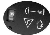
Figure 1 - AC Voltage Switch
