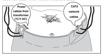
3 Once the cables are connected, insert the Alien 05 into the mounting hole.
