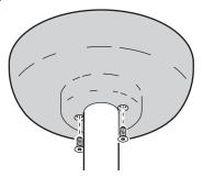
11 Rotate the mounting bracket and tilt the sphere to the correct position and lock them into position using a 2.5 millimeter Allen wrench.
