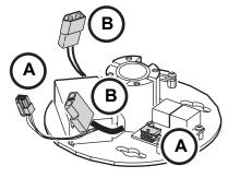
11 Lay the network cables between the 05 Driver/05 Repeaters and the data terminal (A) on the base. See "Laying control network cables" on page 8. Use CAT5 network cables and if the lamp is to be daisy-chained to a subsequent lamp, connect another CAT5 network cable for the link to the
