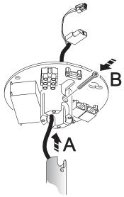
8 Connect the data cable (A) to the data terminal (A). Connect the power connectors (B).
