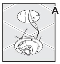
3 Grasp both wire clips (B) simultaneously using both hands and insert the Alien 05 Eyeball into the Halo recessed fixture housing (C and D).
