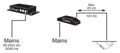
In this configuration the 05 Driver cannot control the supply of power to the Alien 05 luminaires or dim them.
