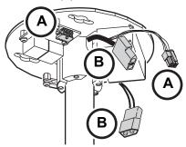
9 If the power and data cables are to pass out through the side of the base cover then remove the three rubber grommets that sit in the cover holes, make a cut in each of them, place them over their respective cables, and push them back into place on the cover.
