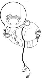
3 If you have attached a 600 mm long arm then attached the cable extension that is supplied to the cable on the Alien 05 Stem Mount head.
