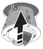
4 Using a 3 mm Allen wrench, tighten the screws to lock the fixture in place. Do not overtighten.
