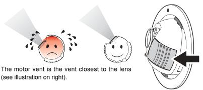
The illustrations below show how to minimize heat stress on the color wheel motor. Down-light installations (a) are straightforward. However, in up-light installations (b and c), ensuring that the motor vent is below the lens, as in (b), will optimize motor cooling.
