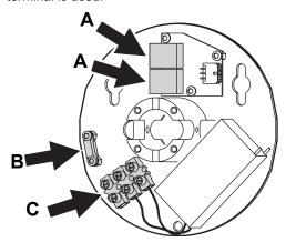
3 Connect the transformer on the Base to power at the terminal (C). See "Connecting transformers to a power supply" on page 11 of this user manual. Anchor the power cable using the clamp (B).
