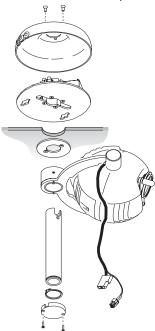
2 Remove the snap ring from the end of the Arm using a pair of retaining ring pliers. Slide the Arm through the hole on the bracket of the Alien 05 Stem Mount head and replace the snap ring.
