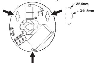
2 Lay the network cables between the 05 Driver/05 Repeaters and the data terminal (A) on the Base. See "Laying control network cables" on page 8. Use CAT5 network cables and if the lamp is to be daisy-chained to a subsequent lamp, connect another CAT5 network cable for the link to the next fixture. Note that it does not matter which network socket on the data terminal is used.
