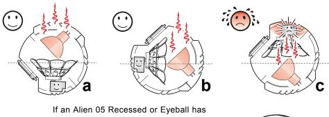
been installed as in (c) above, it can be adjusted to optimize motor cooling by rotating the sphere through 180° (A) and tilting (B) to re-aim the beam.
