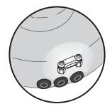
10 Push the base cover up into place and screw it into position using a 2.5 mm Allen wrench.
