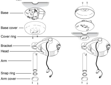
Note that in either configuration that power and data cables can be connected to the base either through the three holes in the side of the Base cover or through the hole in the center of the base.
